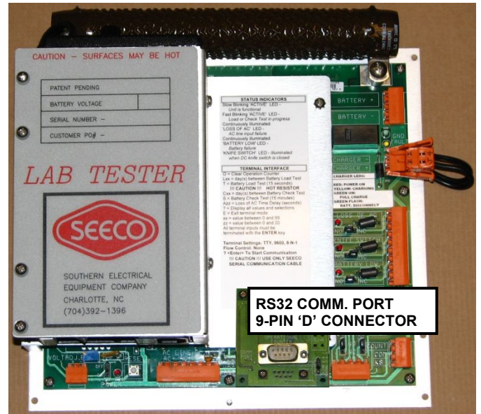
Figure 2 LAB Tester PCB Assembly (shown with optional Operation Counter/Display Board)
