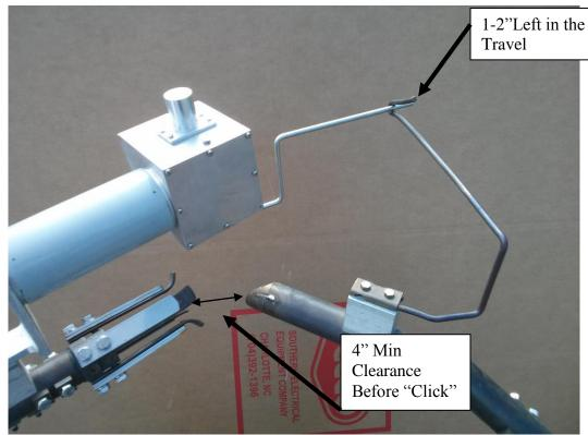
**Image 5. Picture Showing Tripping Position**
